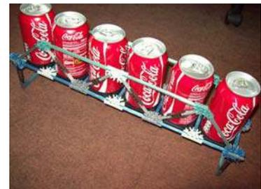
Using the information below, and the algebraic expressions for beam deflection on the previous sheets, work out how thick the beams need to be and find the cheapest price for the floor.
