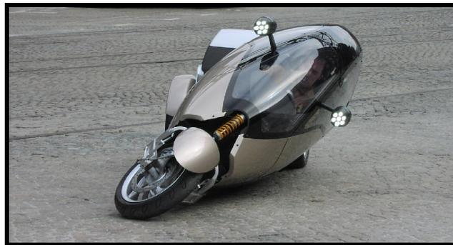
So they developed a tilting mechanism which leans the body of the vehicle like a motorbike at angles upto  $45^\circ$ . This shifts the centre of gravity sideways and pushes the weight on to the inside wheel thus avoiding roll-over. In fact, CLEVER is very clever, and uses a computer control system to work out the best tilt angle, which depends on the speed  $V$  of the car and also on the angle at which the driver steers into the corner as this changes the corner radius,  $R$ .
